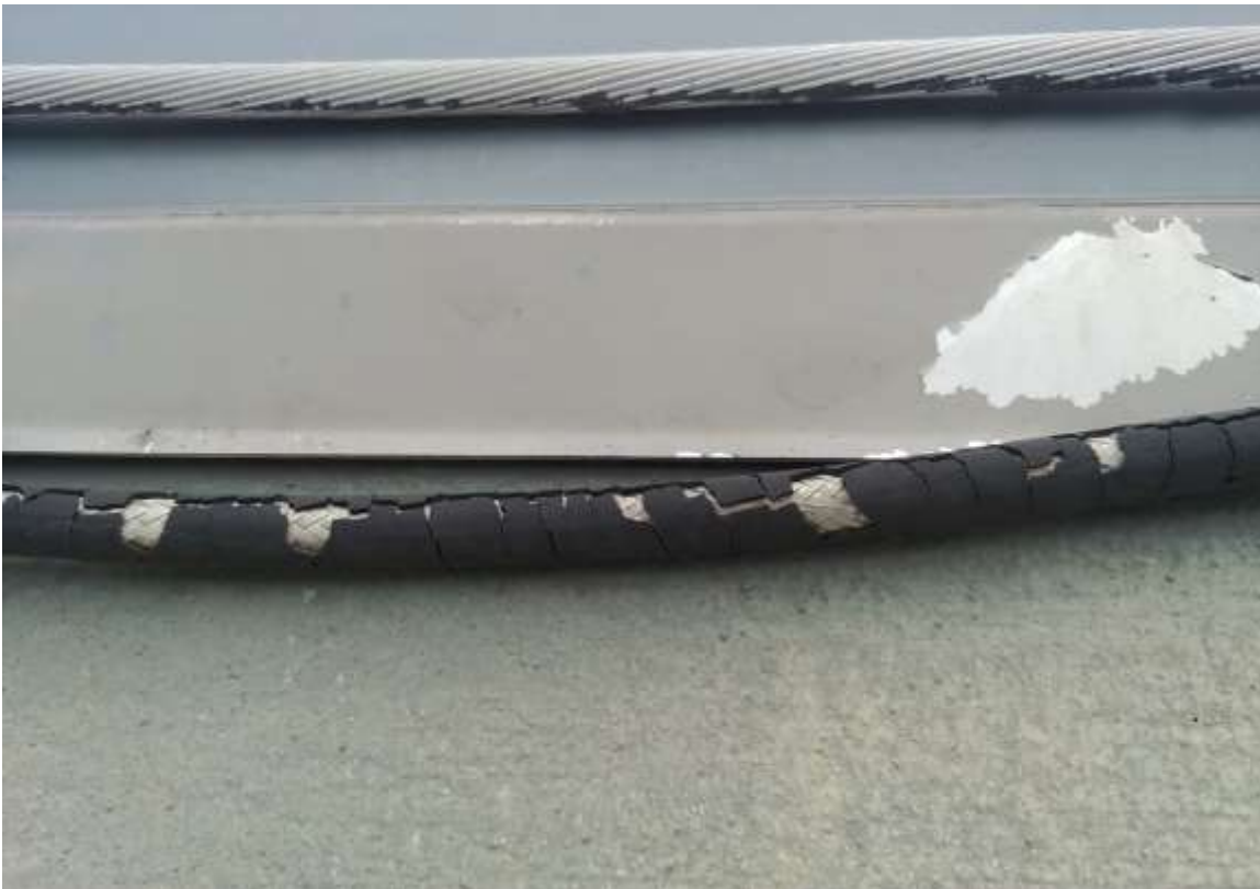
Figure 1: LMR600 Ultra-flex with cracks on the covering
