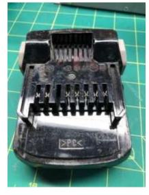
It would be simple just to hook a terminal lug up to the positive and negative terminals of the battery. That did not look to robust to me. A little searching on eBay turned up the following:
